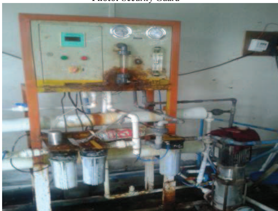
Photo : Reverse Osmosis Process Unit at College of Engineering
