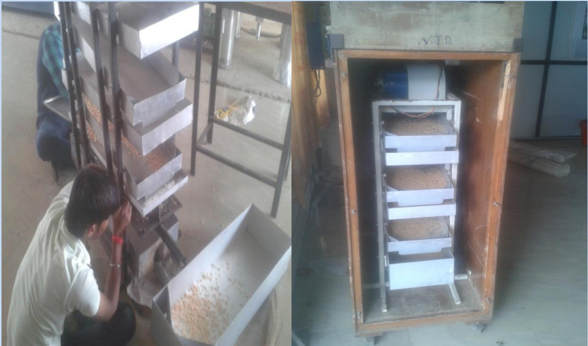
Vibro Thermal Disinfector is provided with Grading and cleaning facility
